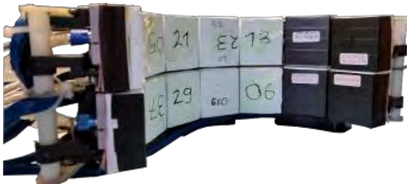
Fig. 8: View on one PET half-ring equipped with detectors.
