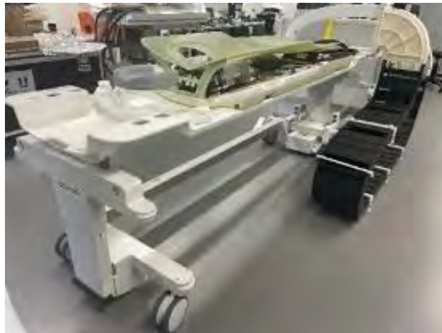
Fig. 7: The figure shows the module mechanics (unpainted) mounted on a commercial patient trolley. The trolley is driven to the MRI with the scanner and the patient as usual and converts the \text{SI}_{1.5} -MRI into a simulated MRI-PET system. The cable management is routed via the cable slapp (black) to the rear end of the scanner, where the power supply unit is located.
