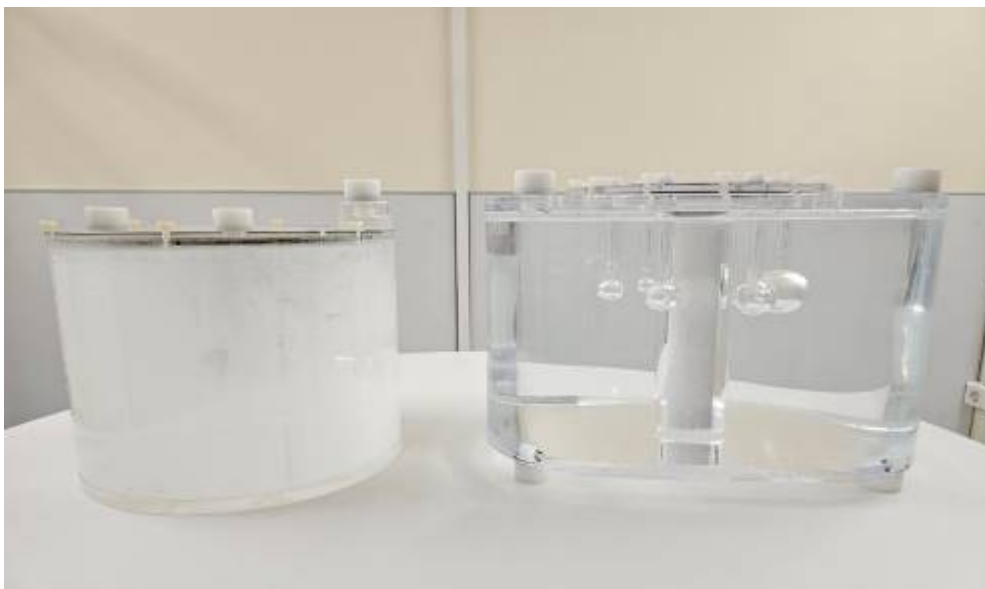
Abb.1: Verwendete Phantome (links: Homogenes Zylinderphantom, rechts: NEMA IEC Body Phantom)
